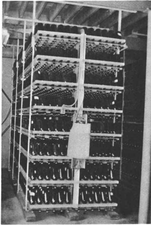
Figure 4. Mechanically operated riddling rack
