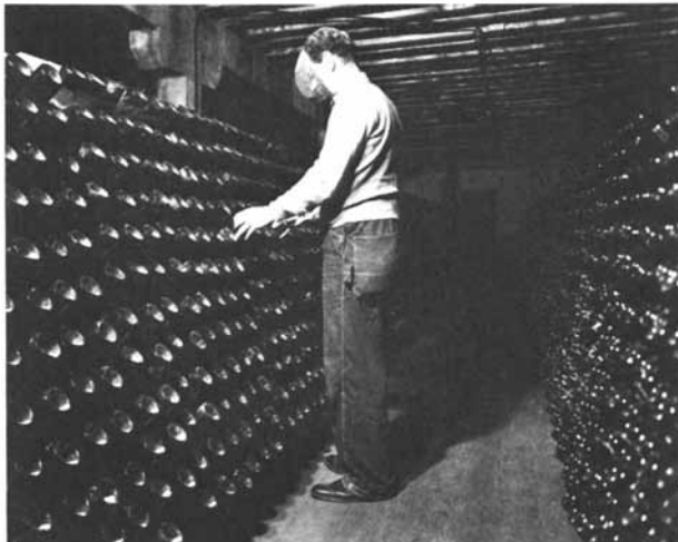
Figure 3. A-frame riddling rack
